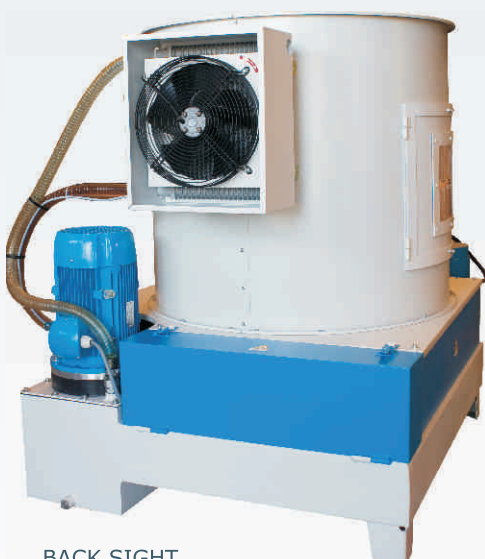
BACK SIGHT New air/oil exchanger (standard)
