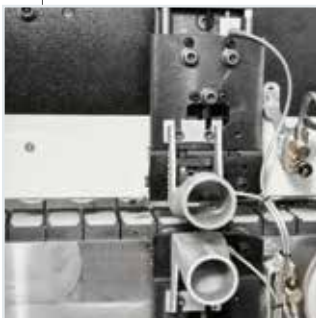
RC-V glue scraping unit: It eliminates any excess of glue in the joint between panel and edge.
