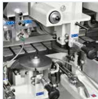
RAS-M edge scraping unit: perfect radius on plastic edges.
