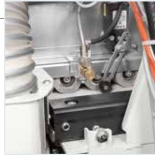
AAL anti-adhesive unit: the highest level of panel cleaning with the application of anti- adhesive spray.
