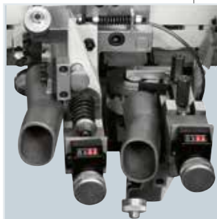
RAS/K edge scraping unit: it eliminates the notches left by the tools on the plastic edges
