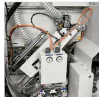
K/SEL end cutting unit: optimal panel finishing thanks to the blade tilting.
