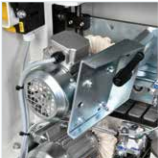
SP-M brushing unit: cleaning and polishing of edge.
