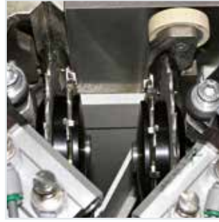
K-2 Radius end cutting unit: cut and radius in a single operation.
