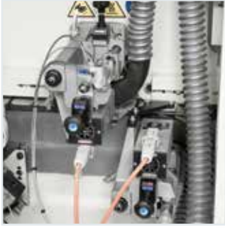
R-K trimming unit: rapid machining changeover between thin, thick and solid wood edges.
