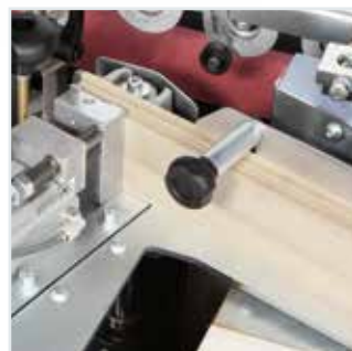
VC-M gluing unit: up to 5 mm thick solid wood edge.
