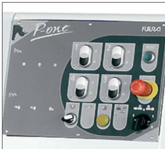
Easy control panel, independent motor starters, 2 feed speeds.
