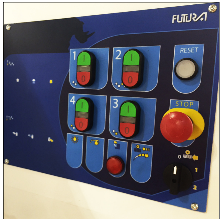
Easy control panel, independent motor starters, 2 feed speeds.
