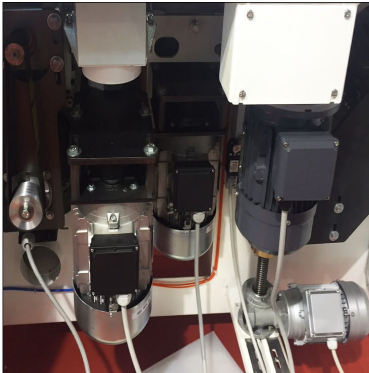
Independent motors to each spindle, poly vee drive belts instead of flat belt, single piece fabricated base.
