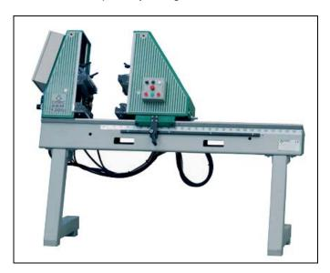
The drawer size can be simply adjusted manually by the operator. Height and width can be adjusted by means of a handle that drives a rack cart for width adjustment and two chain carts for height adjustment. Depth adjustment is obtained by sliding the stroke-pieces along a track that is carved directly onto vises.
