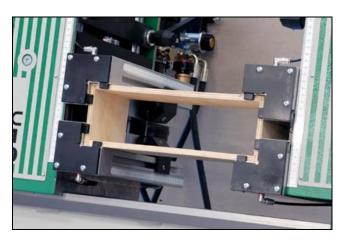
In the discontinuous operating mode, it is possible to hold the crate in the pressing position as long as you wish, so that the operator can easily install the crate's bottom while the crate is still on the machine using the standard riveting systems. In this case, it is the operator's task to control the release of vises through the specially designed pushbutton when the assembly of the crate's bottom is completed.
